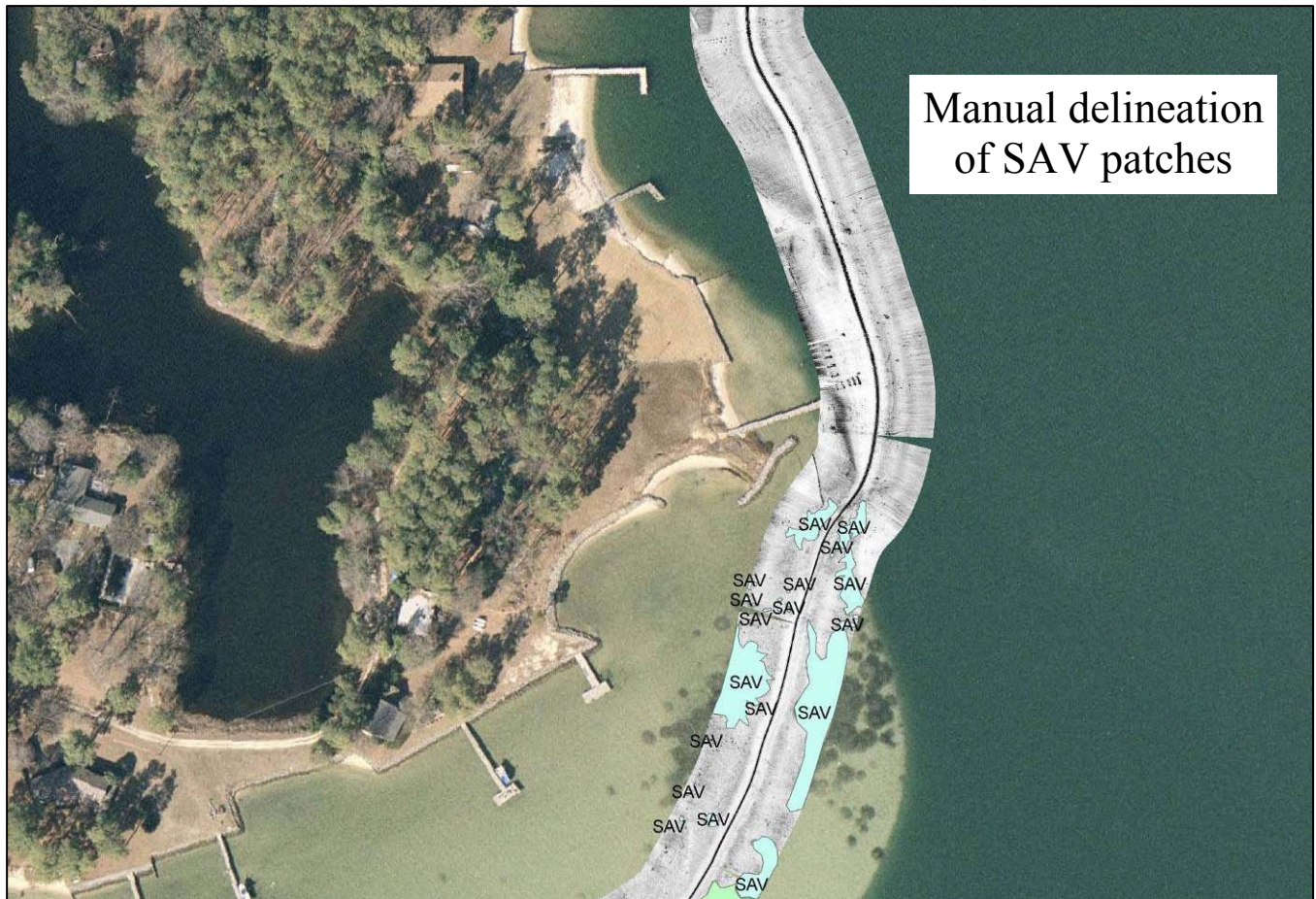
Figure 9. Example of side-scan sonar survey images with manual delineation of structural subtidal habitat, such as submerged aquatic vegetation (SAV). Delineated areas were converted to polygon shapefiles for further analyses. Digital data are available on the DVD: Piankatank River Nearshore Seabed Classification.
